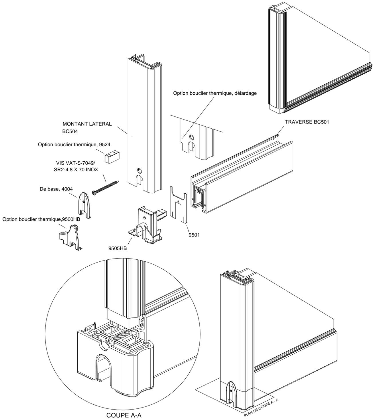
DRAINAGE ET EQUILIBRAGE DE PRESSION CADRE OUVRANT
