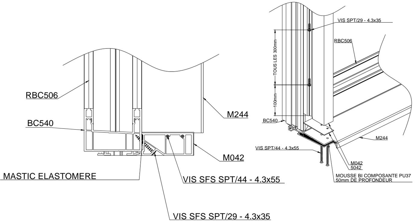
ASSEMBLAGE CADRE OUVRANT MONTANT DE TETE - TRAVERSE
