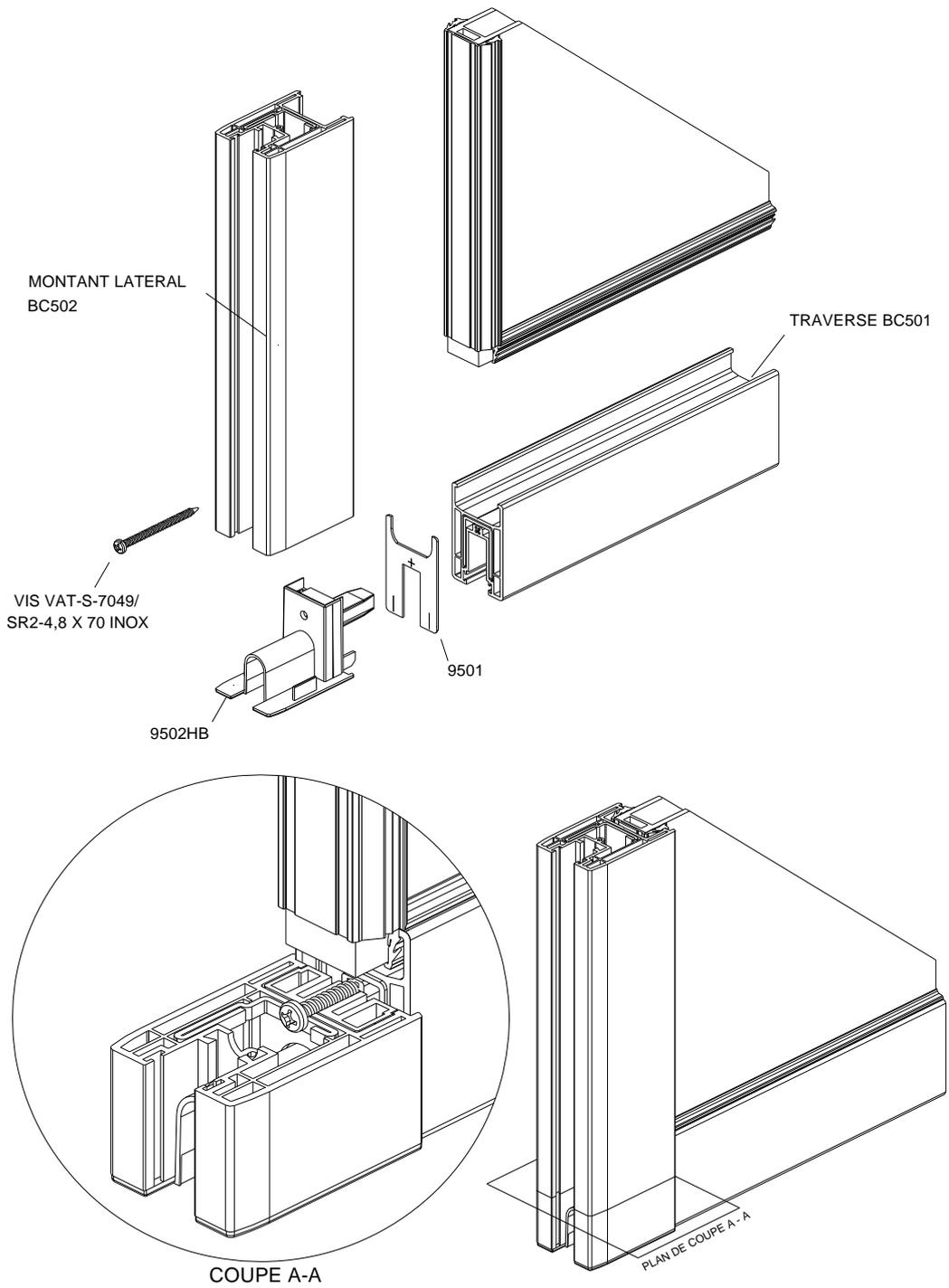
ASSEMBLAGE CADRE OUVRANT CHICANE INTERIEURE - TRAVERSE
